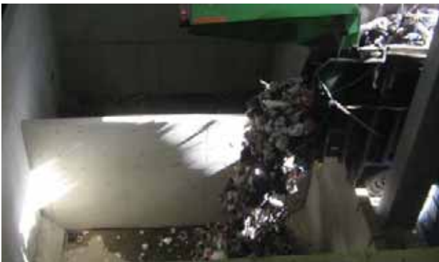
1 Waste being deposited into the Bio-MRF from the back of household refuse collection vehicle
