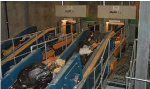
2 Waste entering the Opti-Bag system in order to separate orange bags containing recycling materials
