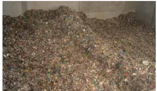
5 Shredded Residual Waste during maturation in Bio-MRF
